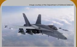
Fig. 1 Royal Canadian Airforce CF18M Armed Fighter Jet, service ceiling of 48,000 feet altitude and can reach MACH 1.8 and fight up to 7.5G.
